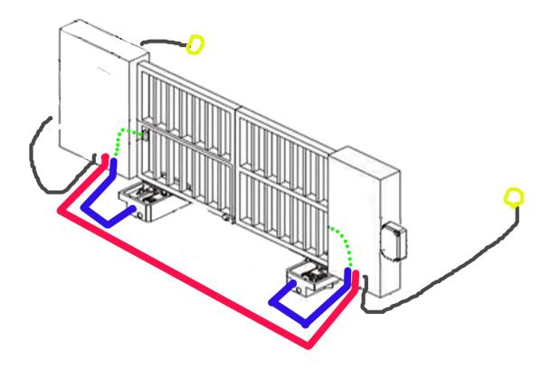
····· Duct in pillars from photocells
